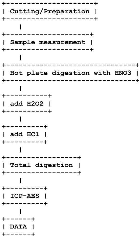
The samples were dissolved totally by pre-conditioning method according to above flow chart.
